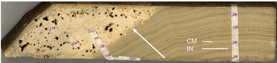
Fig. 6. Sample dating from 1759 to 1853, taken during the 2009 renovation of the Harris House, Aurora, Indiana. Photograph 2023. Tulip poplar sapwood is more susceptible to decay and insect damage than heartwood; this floor joist sample required sawing a cross section because coring would have resulted in broken, undatable sapwood fragments.
