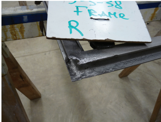
Fig. 2. Severe corrosion requiring new steel, 2011.
