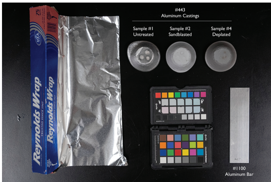
Fig. 11. Post-experiment color differences between Samples 1, 2, and 4, with other aluminum objects included for comparison. Photograph by Preston Hull, 2024.
