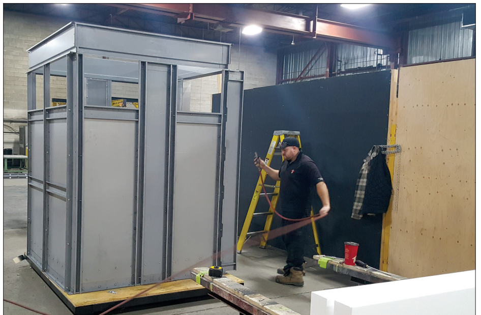
Fig. 8. Mock-up of the reproduction elevator cab in the factory. The walls consist of formed panels of cold-rolled sheet steel bolted together.
