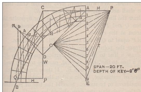
**Fig. 8.** Frank Kidder's construction of thrust line for a symmetrically loaded semicircular arch from *The Architect's and Engineer's Pocket Book*, 3rd ed. (New York: John Wiley and Sons, 1886).
