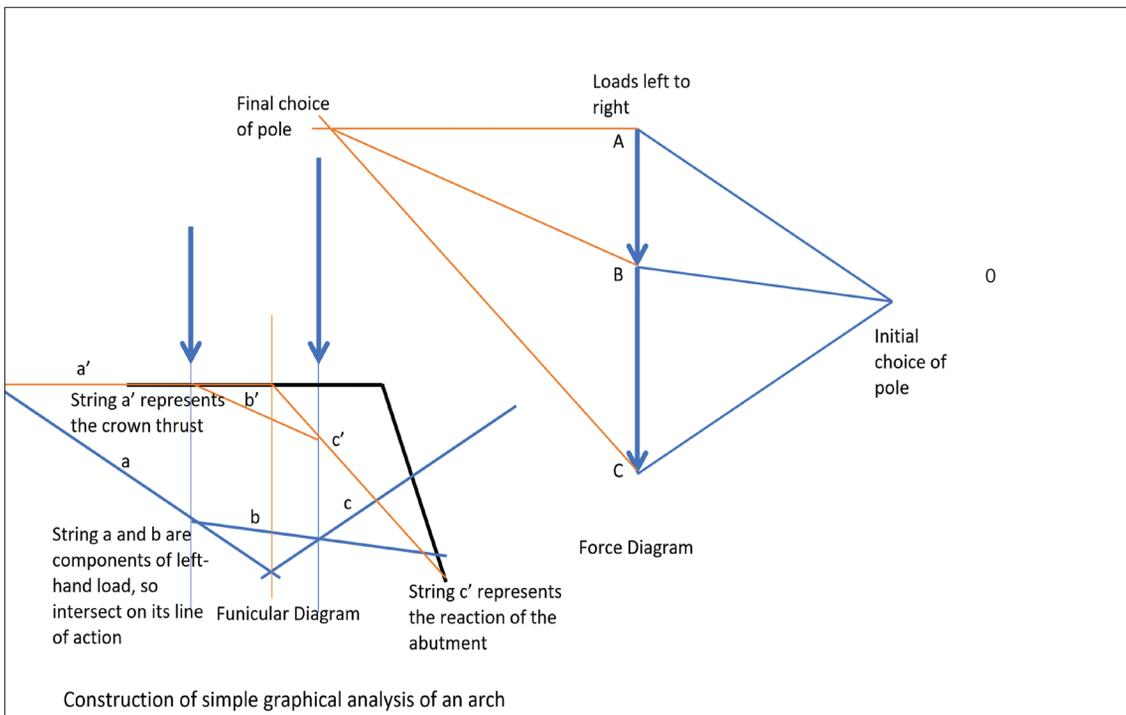
**Fig. 7.** Simplified application of graphical analysis for a symmetrical half-arch. Figure by Karissa Shaner.
