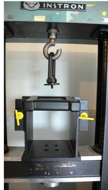
Figure 3.7: Instron machine with testing frame
