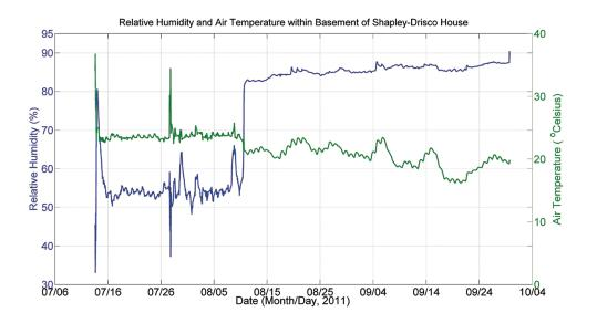
Fig. 7. Relative humidity and air temperature measured within the basement of the Shapley-Drisco House from July 2011 to October 2011.
