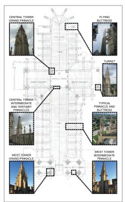
Fig. 5. Plan showing damage distribution.
