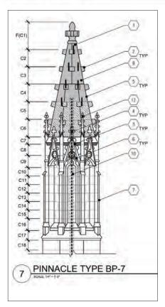
Fig. 9. Damage legend showing typical damage nomenclature generated after cathedral-wide assessment.
