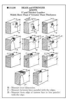
Fig. 5. Instructions for measuring knots on beams and stringers. Courtesy of Western Wood Products Association.
