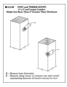
Fig. 6. Instructions for measuring knots on posts and timbers. Courtesy of Western Wood Products Association.
