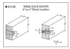
Fig. 4. Instructions for measuring knots on 2inch- to 4-inch-thick lumber, which includes structural joists and planks. Courtesy of Western Wood Products Association.
