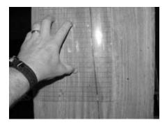
Fig. 9. The use of a 1/2-inch grid on acetate for measuring slope of grain.
