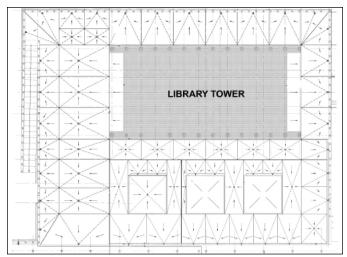
Fig. 3. Plan of the LBJ Library plaza at the subsurface (waterproofing) level, showing the slope of the new bonded overlay added atop the original structure. Each rectangular area is drained to an individual drain body.
