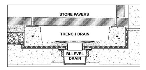
Fig. 6. Section detail at new perimeter trench drain at the LBJ Library plaza, showing a pedestal-set paver atop precast-concrete trench unit. Within the precast concrete trench, bi-level drain bodies were used.
