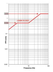
Fig. 4. "Safe limit" to prevent threshold cracking in plaster walls. From USBM RI 8507 and John F. Wiss, "Construction Vibrations," (1981): 167-181.
