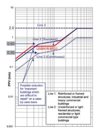
Fig. 5. Vibration limits recommended by BS 7385-2 superimposed on the USBM RI 8507 limit.
