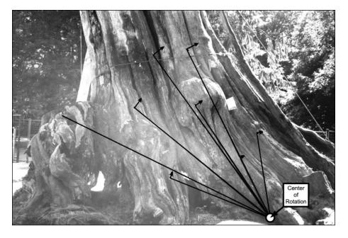
Fig. 6. This 2008 photograph shows the unstabilized position of the Hollow Tree, and the lines and arrows show the movement of the tree that resulted from the test displacement. Image by Lorne Whitehead.
