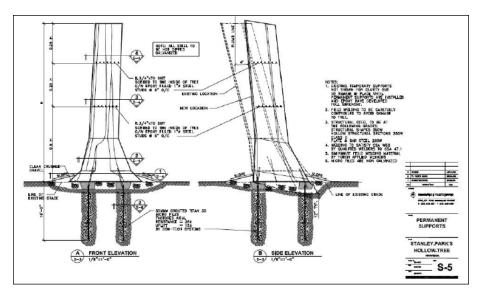
Fig. 7. Sections showing the micropiles, concrete pile cap, and major support frame, 2009. Drawing by Cascade Engineering.
