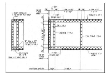
Fig. 6. Lobato Bridge, detail from the design drawings of the end of a girder. Efforts were made to replicate the historic appearance as much as possible within the confines of the project's design criteria. Compare the connections using tension controlled bolts to the original arrangement of rivets shown in Figure 3. Drawing by HDR.
