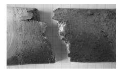
Fig. 5. Specimen, lacing bar after testing in tension failure. Photograph by the author.
