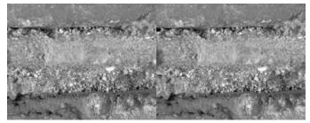
Fig. 9. Stereo images of the eroded Indiana limestone, with visible fossil fragments.
