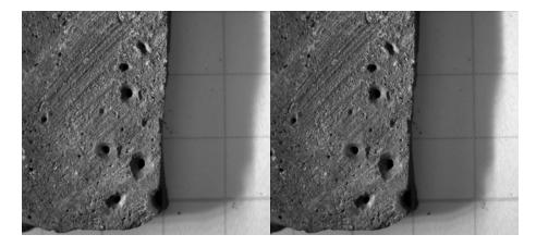
Fig. 8. Stereo images of a capping-compound fragment. Note the difference in shadow length on the right side of the fragment shown in each image, which makes it possible to determine the thickness of the fragment.
