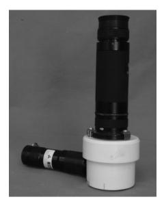
Fig. 4. The field microscope with a light-shroud base and low-angle lighting.
