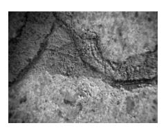
Fig. 3. The vertical surface of weathered dimensional limestone. The photograph was taken with the field microscope and camera shown in Figure 2, using natural, low-angle lighting. The width of the field of view is 3/16 inch.
